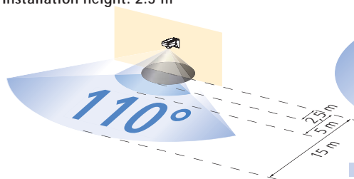
SPHINX 105-110 detection range Installation height: 2.5 m
